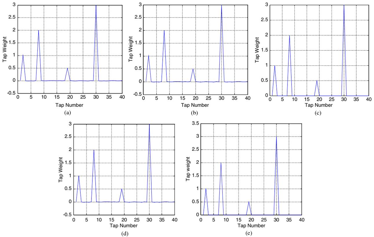
**Fig. 13.** (a) Estimated channel impulse response by the standard RLS algorithm for white input. (b) Estimated channel impulse response by the standard RLS algorithm for colored input. (c) Estimated channel impulse response by the RLS algorithm with ADG for white input. (d) Estimated channel impulse response by RLS algorithm with ADG for colored input. (e) Estimated channel impulse response by the RLS algorithm with TD for colored input.
