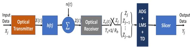
**Fig. 3.** OWC system implementing LMS channel estimation algorithm based on ADG with TD.
