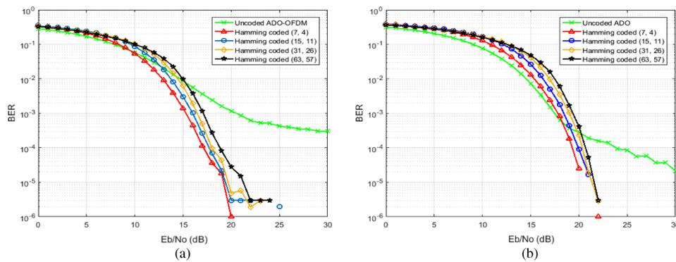
**Fig. 5.** BER performance for the uncoded ADO-OFDM system and the Hamming coded system with different coding rates at DC bias: (a) 3 dB and (b) 7 dB.
