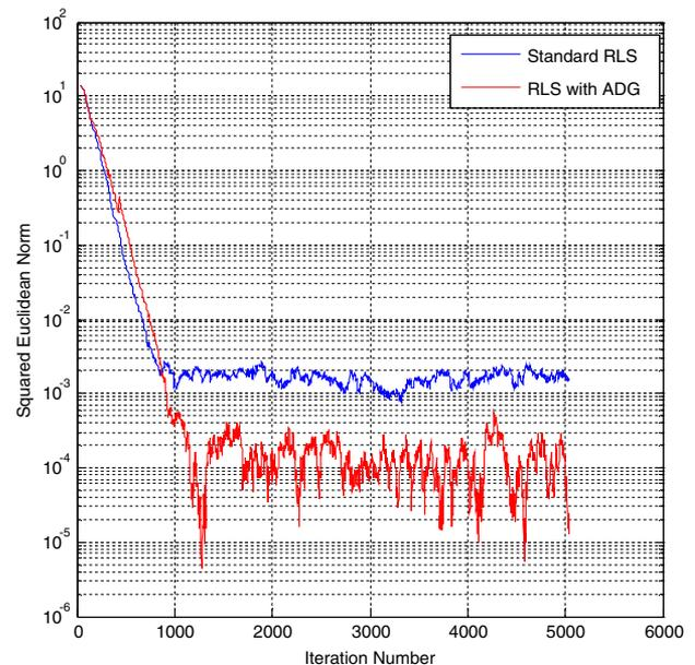
**Fig. 14.** Asymptotic behavior for the standard RLS algorithm and the RLS algorithm with ADG for white input.
