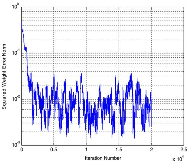
**Fig. 10.** Squared weight-error norm performance using LMS algorithm with ADG and TD.
