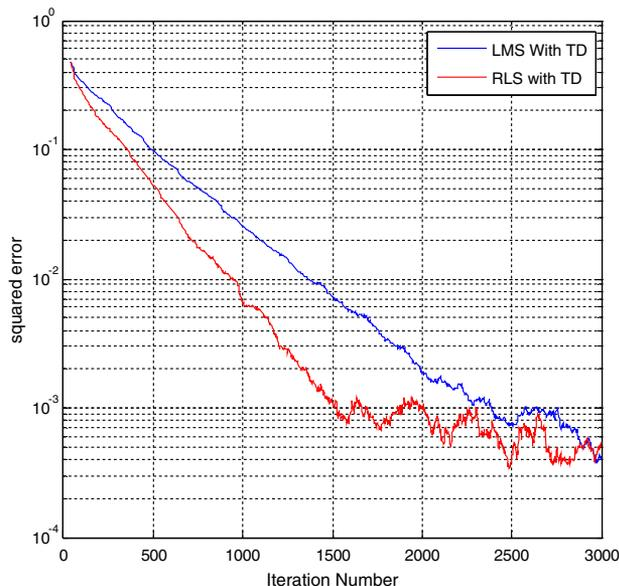
**Fig. 20.** Squared weight-error performance of the LMS algorithm with ADG and TD and the RLS algorithm with ADG and TD.
