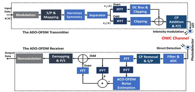
Fig. 2. General block diagram for the ADO-OFDM technique [18].
