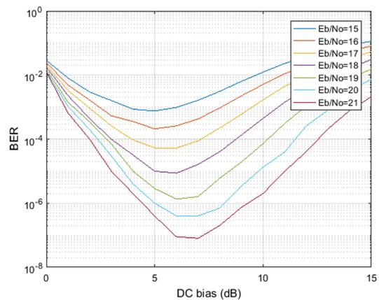
**Fig. 4.** BER versus DC bias (dB) with different values of  $\frac{E_b}{N_0}$  (dB) showing the optimal DC bias value and the corresponding BER.
