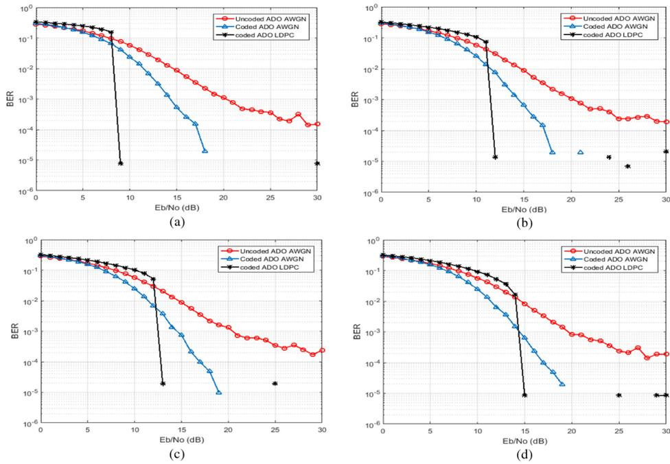
**Fig. 7.** BER performance comparison between Hamming coding and LDPC coding at a DC bias of 3 dB with different coding rates: (a) 1/2, (b) 3/4, (c) 4/5, and (d) 8/9.
