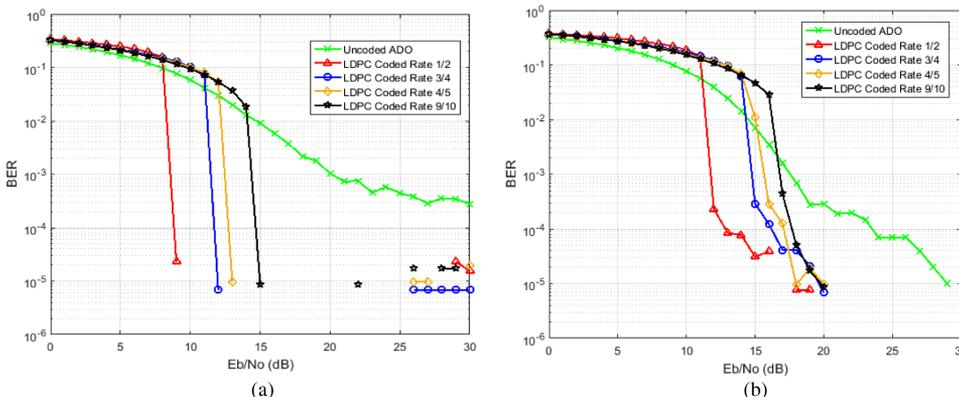
**Fig. 6.** BER performance for the uncoded ADO-OFDM system and the LDPC coded system with different coding rates at DC bias: (a) 3 dB and (b) 7 dB.
