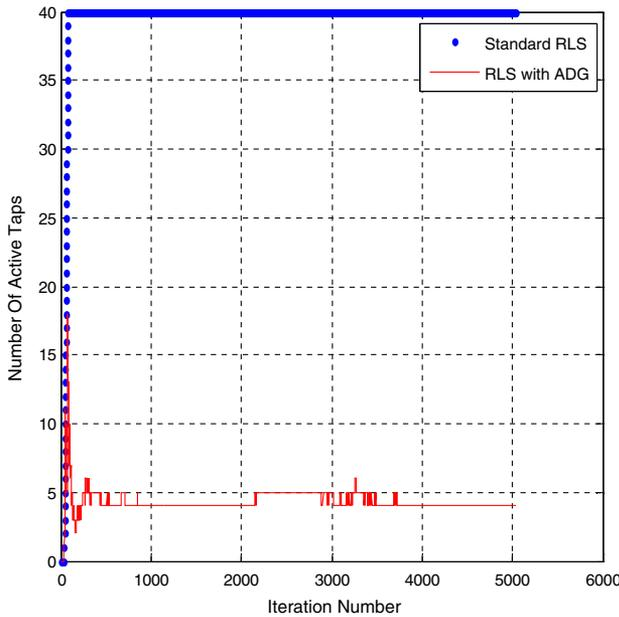
**Fig. 16.** Estimation of the number of active taps by the standard RLS algorithm and the RLS algorithm with ADG for white input.
