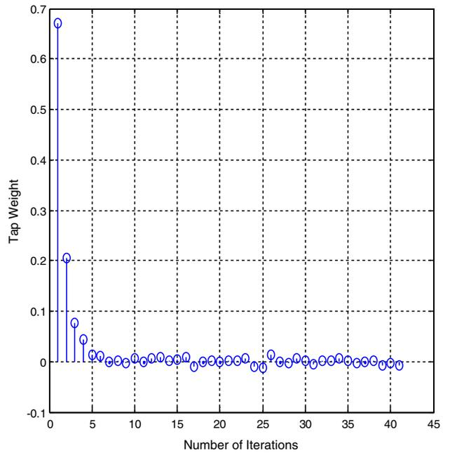
**Fig. 18.** Estimated channel impulse response using the standard RLS algorithm.
