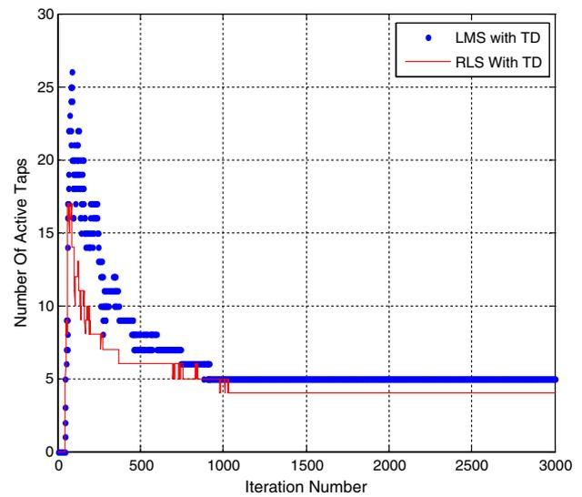
**Fig. 21.** Estimated channel taps using the LMS algorithm with ADG and TD and the RLS algorithm with ADG and TD.
