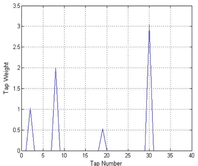
**Fig. 12.** Supposed impulse response of the multi-tap channel.
