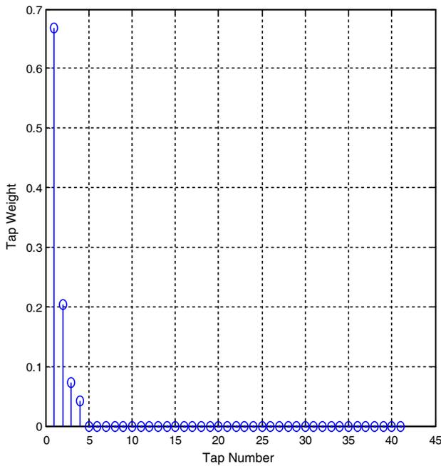
**Fig. 19.** Estimated channel impulse response using the RLS algorithm with ADG and TD.
