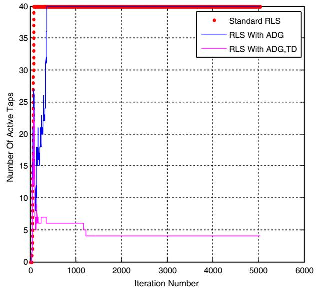
**Fig. 17.** Estimation of the number of active taps by the standard RLS algorithm, the RLS algorithm with ADG, and the RLS algorithm with ADG and TD for colored input.
