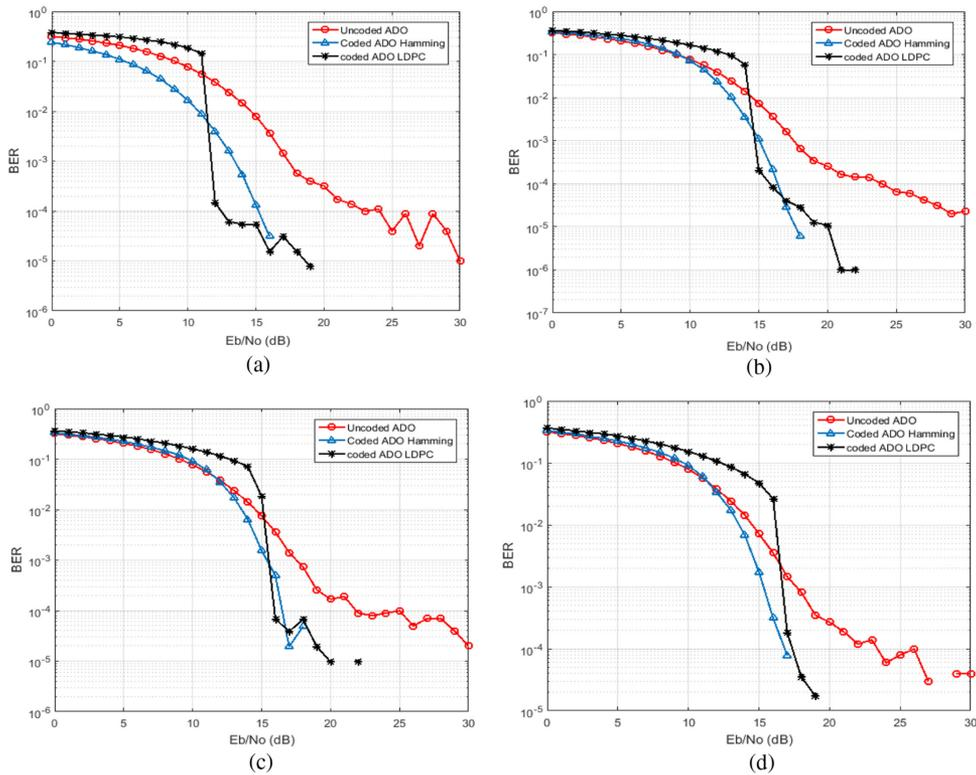
**Fig. 8.** BER performance comparison between Hamming coding and LDPC coding at a DC bias of 7 dB with different coding rates: (a) 1/2, (b) 3/4, (c) 4/5, and (d) 8/9.
