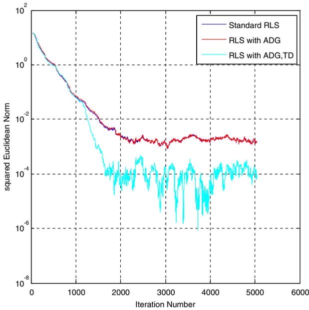
**Fig. 15.** Asymptotic behavior for the standard RLS algorithm, the RLS algorithm with ADG, and the RLS algorithm with ADG and TD for colored input.
